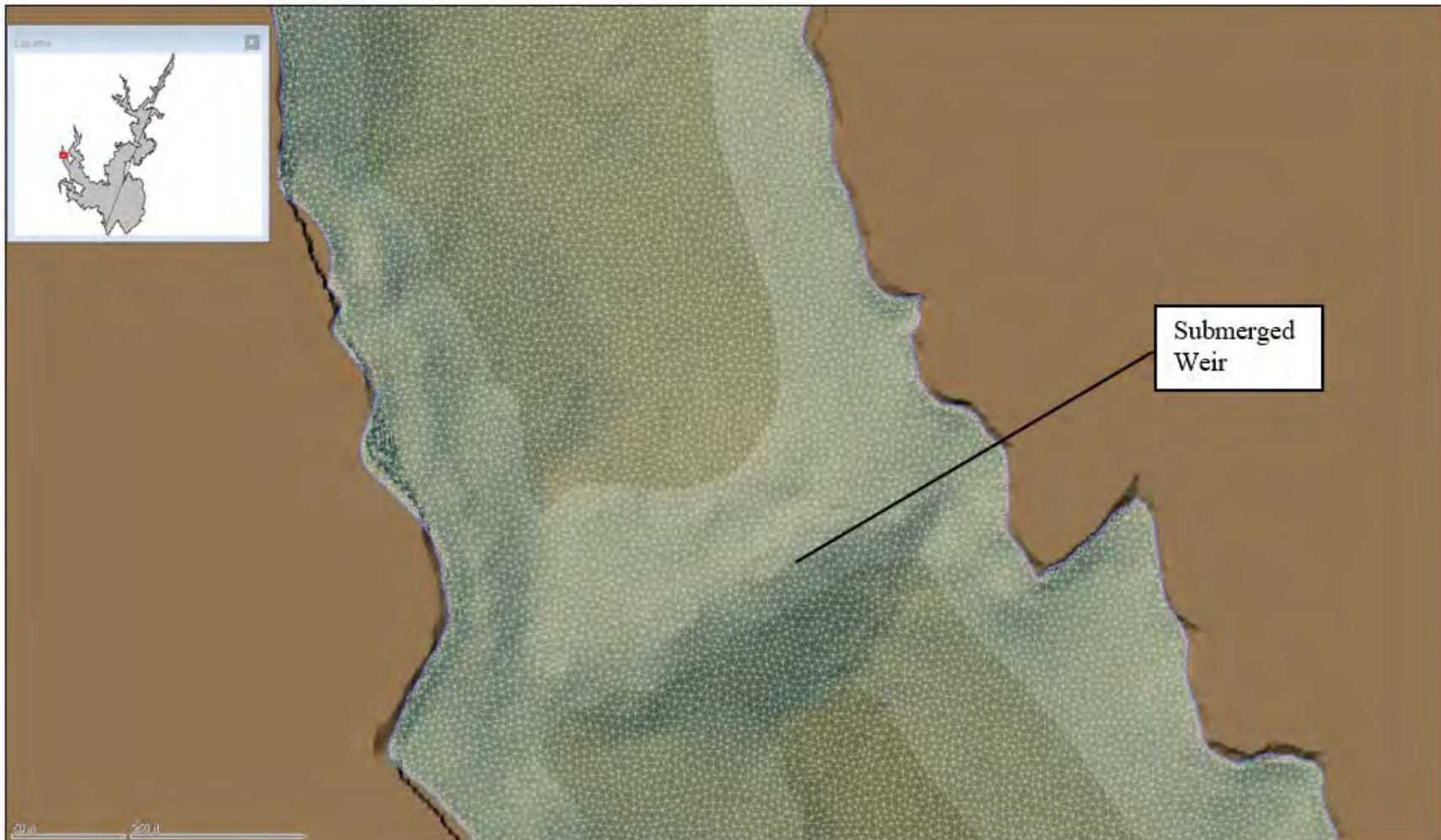
Figure 4-4. Example of 2-D Model Mesh Section
