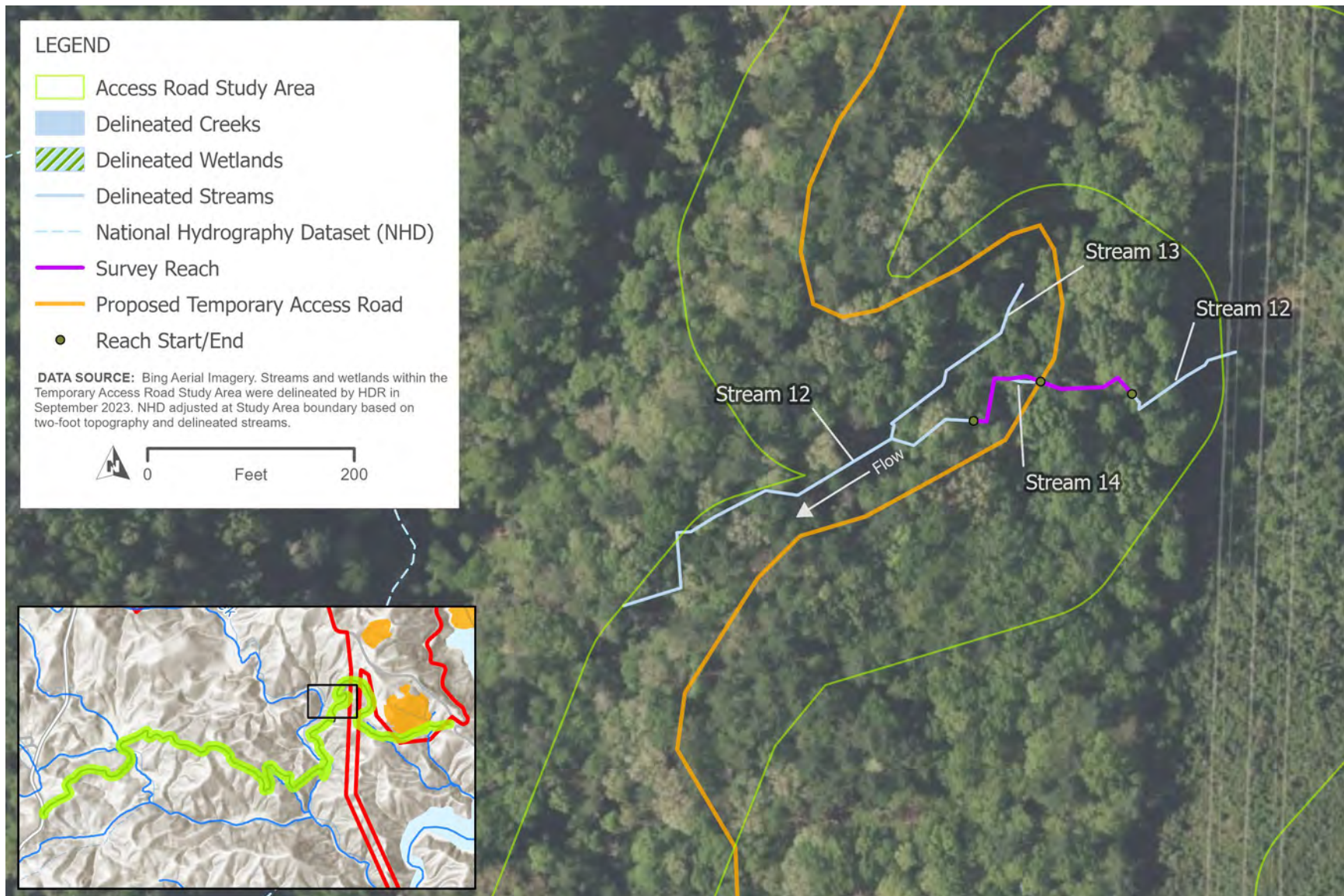
Figure 4. Streams and wetlands surveyed along the proposed temporary access road at the Stream 12 crossing
