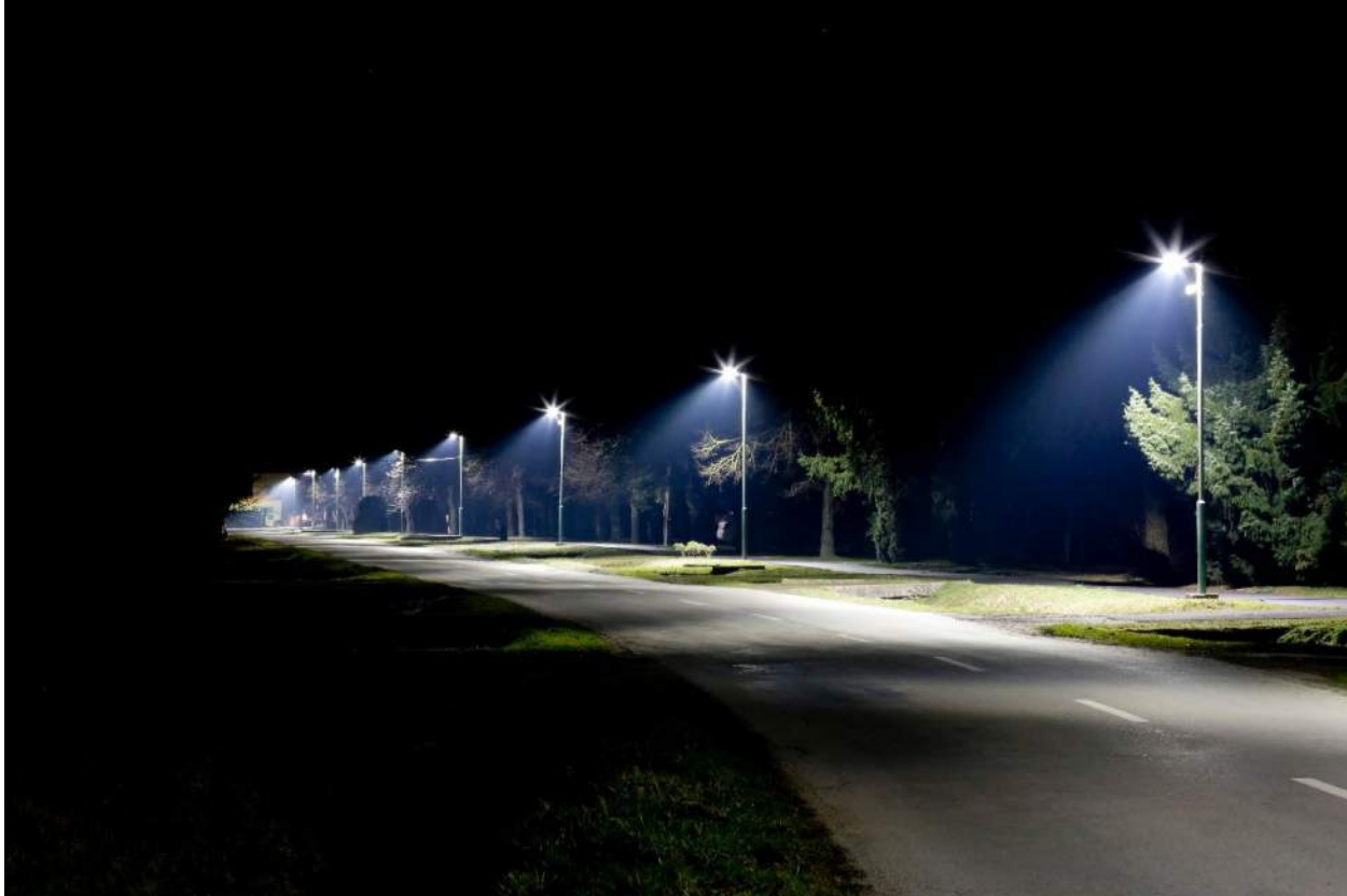
Figure 6-38. Example of Fully Shielded Streetlight Fixtures
