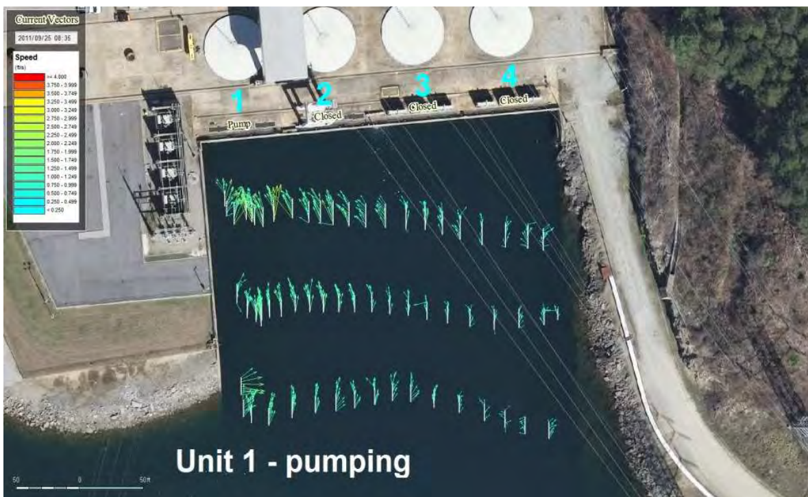
Figure 19a. Individual velocity profiles in the JPSS Tailwater with one unit pumping.
