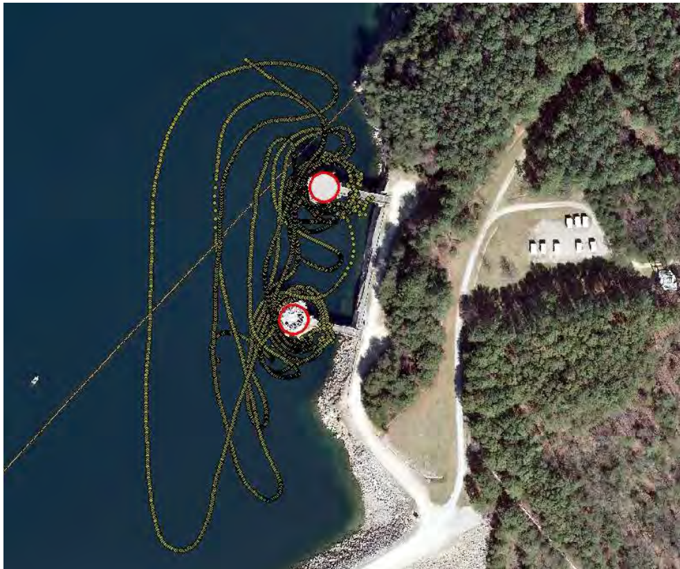
Figure 10. Example of boat track (GPS points during 4 Unit Operations) during data collection at JPSS Intakes.
