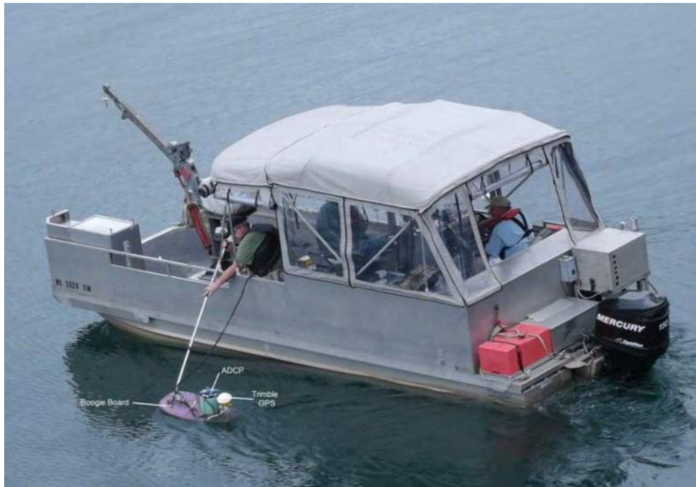
Figure 9. RD Instruments Rio Grande 600 kHz ADCP and GPS mounted on a boogie board.
