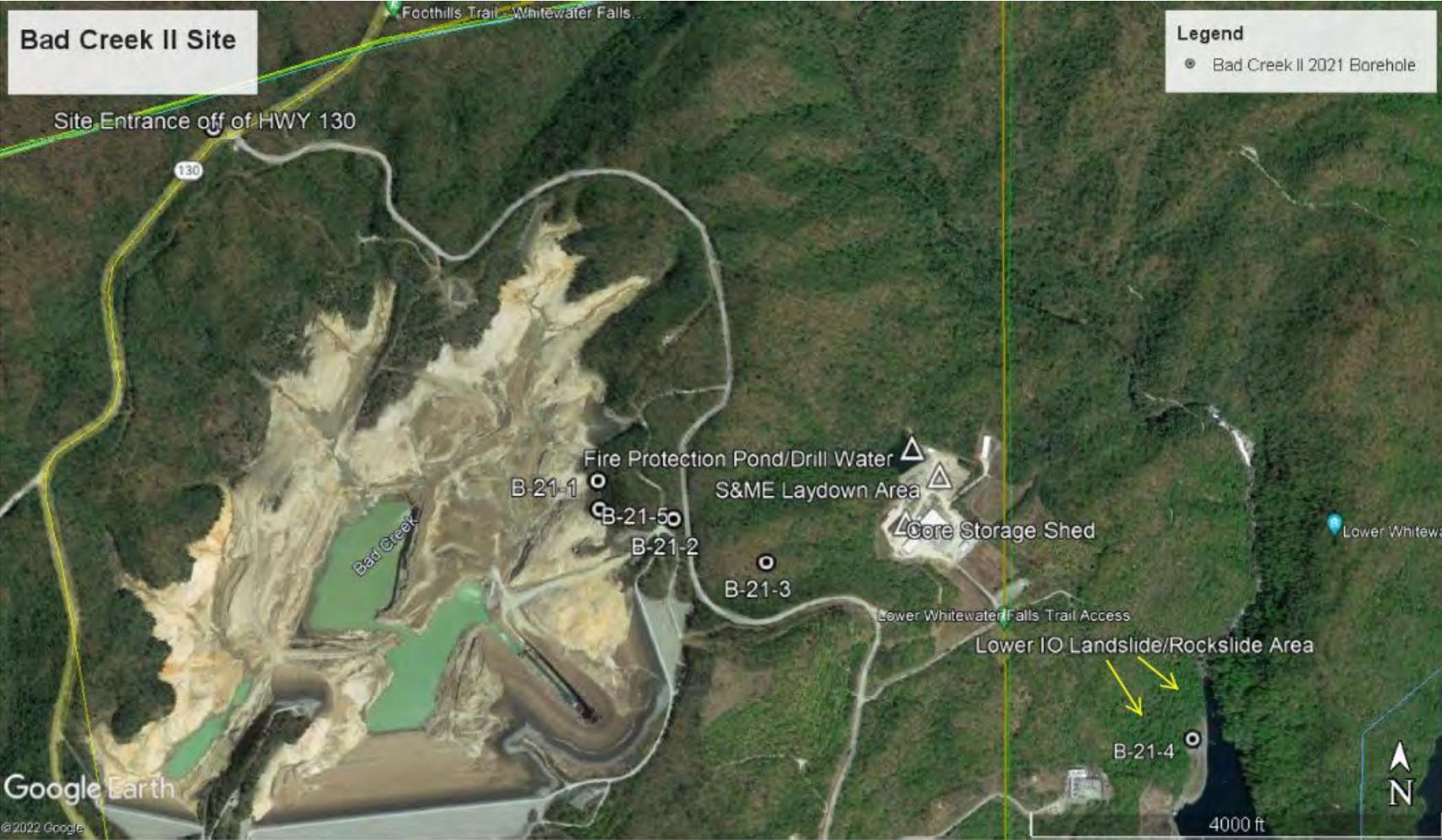
Figure 1. Bad Creek II Geotechnical Investigation General Site Features Geotechnical Drilling
