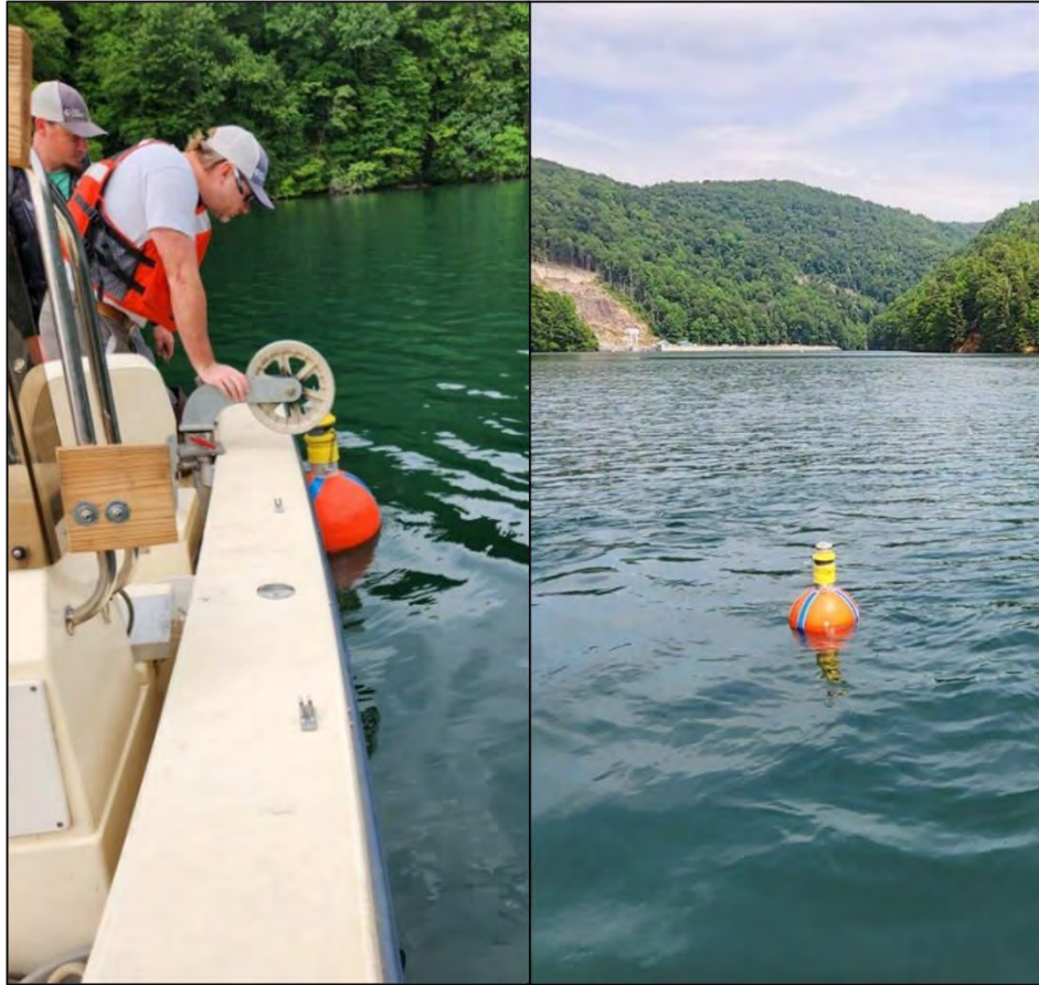
Figure 5-2. Instrumentation Deployment with Boat-mounted Winch (left) and Deployed Water Quality Monitoring Buoy and Datalogger Chain at Station 564.0 (right)
