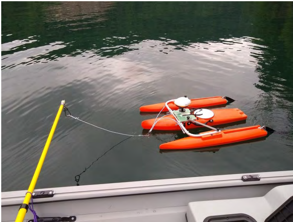
Figure 4-4. Teledyne RDI RiverRay ADCP and Trimaran
