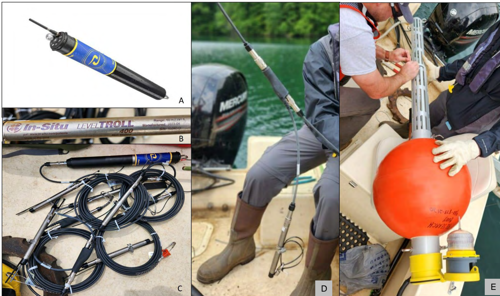
Figure 5-1. Water Quality Instrumentation: (A) VuLink device; (B) In-situ datalogger; (C) VuLink device and dataloggers on single continuous cable system; (D) Deploying stainless steel cable with dataloggers; (E) High visibility buoy with protective cage for VuLink device
